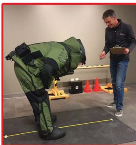
Figure 5: NIJ Dynamic FOV test – Head and Body motion with volunteer
