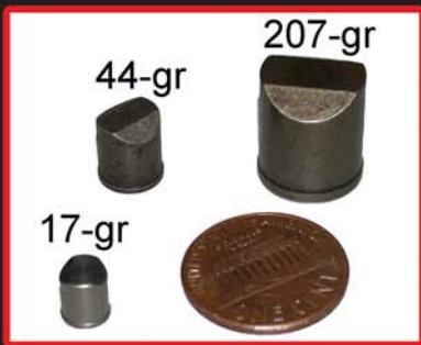
Figure 1: NIJ 0117.01 Fragment Simulating Projectiles (17, 44 and 207-grain)
