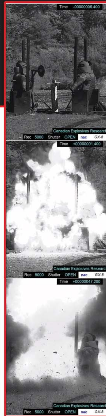
Figure 2: High speed video images of the NIJ 0117.01 blast overpressure test. Kneeling facing 1.25 lbs (0.567 kg) of C4 explosive, at a standoff of 2 feet (0.6 m). Two mannequins used for more data
